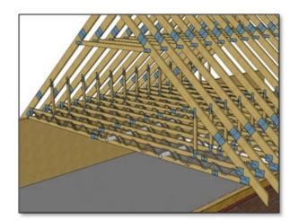
Combining the solid feel of a MiTek Posi-Joist™ with the benefits of a conventional attic truss, the MiTek Posi-Attic enables you to span further than ever before.
