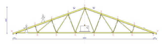
Any compression member, such as the top chord of a trussed rafter, when subject to load, will deflect in both the vertical and horizontal planes. When the deflection is about the minor axis it is usually referred to as buckling.
